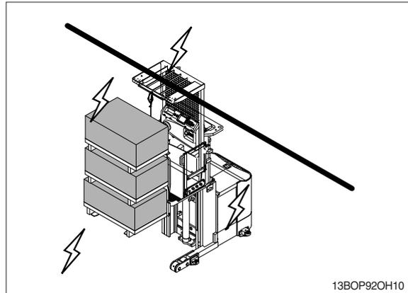
⚠ If the machine touches the electric power lines, keep standing in the operator's compartment and make sure the personnel on the ground do not touch the machine until turning off the electric current.
